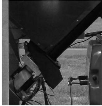
**Reduction motor:** if the motor stops for signaling **"ALAR-DEP-FAIL"** or **"ALAR-SIC-FAIL"** the boiler continues to function until the flame goes out for lack of fuel, and until it has cooled down to the minimum level.
