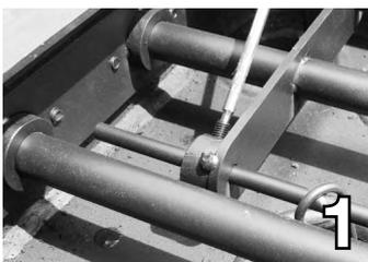
The operation should be completed by unscrewing with a screwdriver the fixing bushings (photo 1). Remove the screws holding the cleaning kit to the camera body and pull it completely (photo 2-3).
