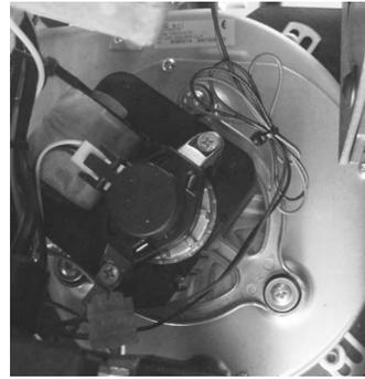
**Flue gas temperature sensor:** thermocouple that measures the temperature of the fumes while keeping the operation or shuts the boiler when the flue gas temperature drops below the preset value.
